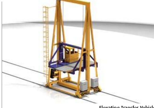
Elevating Transfer Vehicle - 20ft NEP
