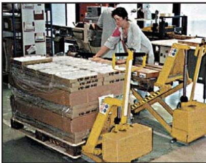
*For high maneuverability in narrow aisles and minimum reach-over using open bottom skids or pallets.*
