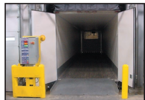
▲ Conventional pit-style designs allow interior energy to escape and outside air infiltration through the pit, compromising efficiency and increasing the risk of spoilage.
